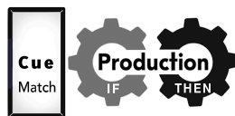
Figure 1: Production rules are formatted as a condition-action pairing. IF the condition side matches to the cue in working memory, THEN it fires an action.
